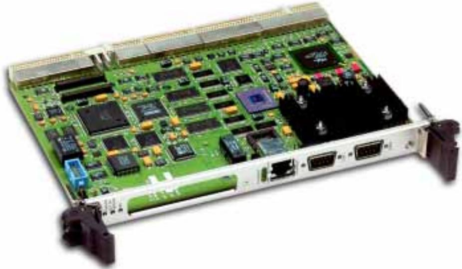
*Denali*™ is a 6U cPCI board with PowerPC 603e @ 200MHz processor (optional PowerPC 740 @ 266MHz). The board has 64 Mbyte of SDRAM, 8 Mbyte of flash memory, 512Kbyte socketed flash, 10BaseT/100BaseTX ETHERNET with interface on an RJ-45 connector, 32K byte NVRAM/RTC, two RS-232C ports with interface to DB-9 connectors, PMC interface, ATM SAR with dual J5 interfaces, PCI bridge to cPCI bus, watch dog timer, and interface to 8 digital I/O signals.
