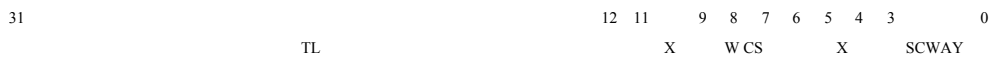
Figure 7-50 The format when the TagLo register is used to access the D-Cache Tag
