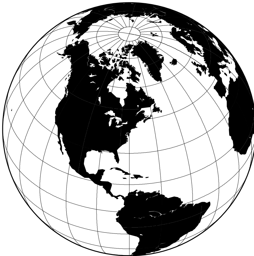
Figure 6.11: Hemisphere map using the Orthographic projection.
