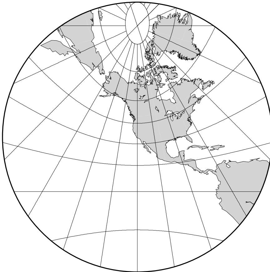
Figure 6.13: Gnomonic azimuthal projection.
