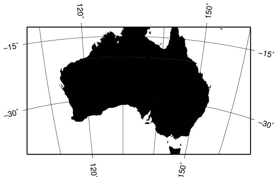
Figure 6.9: General stereographic conformal projection with rectangular borders.
